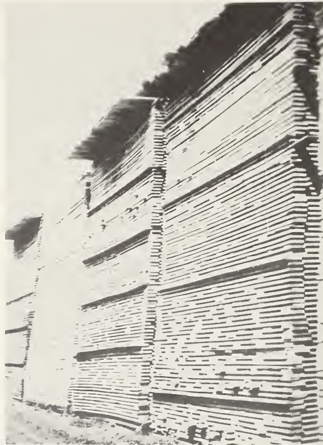
Figure 37. --Drip boards at the rear end of a pile.
